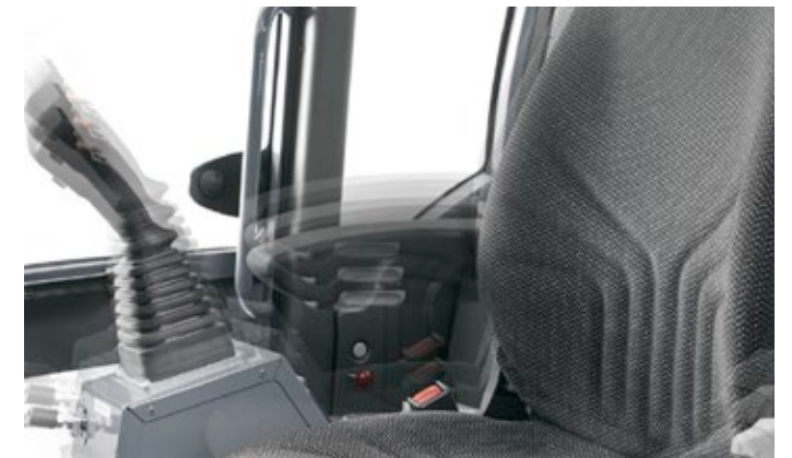
Adjustable joystick console on the operator's seat that swings along.
