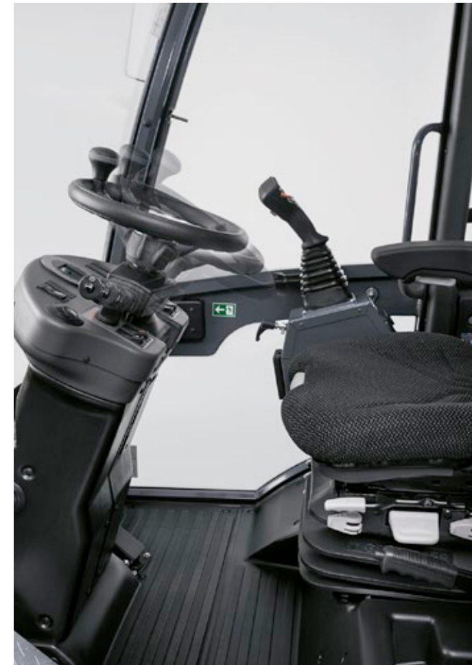
Comfortable work: adjustable steering wheel and air-cushioned comfort seat (optional).
